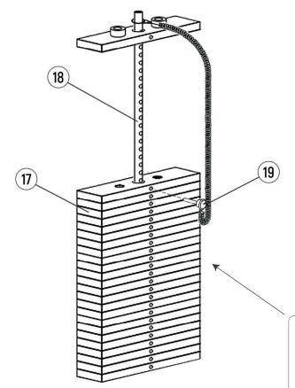
See 6 Step Weight Stack Assembly Directions, starting on Page 17, for Weight Stack Assembly Details
